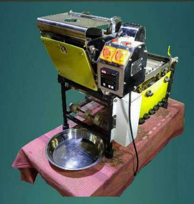
THIS IS NEW DESIGN FROM ROTILAA. VERY COMPACT, TABLE TOP MODEL. VERY LIGHT IN WEIGHT. EASY FOR PORTABILITY AND DYNAMIC IN PRODUCTION. ROTI SIZE IS 8" DIA MAXIMUM. THICKNESS CAN BE SET AS PER REQUIREMENT.
